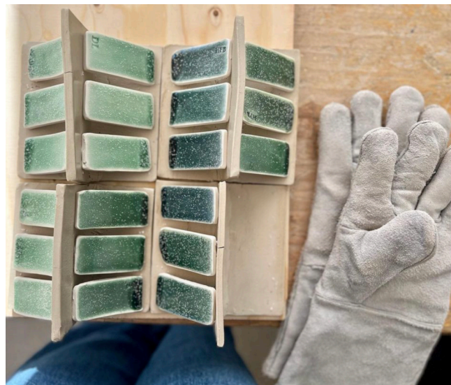
Fig.12, Testing glazes made from langoustine remains, 2022, by Wathne, https://www.instagram.com/p/CcvR3nsDU9/?hl=de
